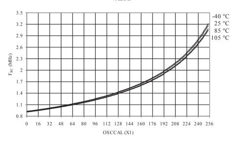
Figure 33-46 Calibrated 1MHz RC Oscillator vs. Temperature
