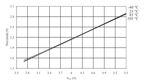
Figure 33-26 Reset Pin as I/O - Input Threshold vs. V<sub>CC</sub> (V<sub>IL</sub>, I/O Pin Read as '0')
