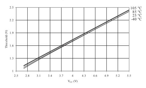
Figure 33-24 I/O Pin Input Hysteresis vs. V<sub>CC</sub>
