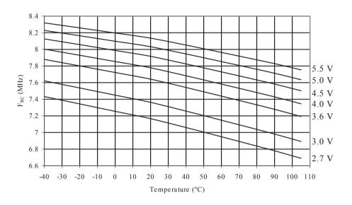
Figure 33-38 Calibrated 8MHz RC Oscillator vs. V<sub>CC</sub>
