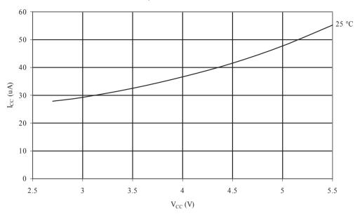
Figure 32-20 Standby Supply Current vs. V<sub>CC</sub> (4MHz Resonator, Watchdog Timer Disabled)
