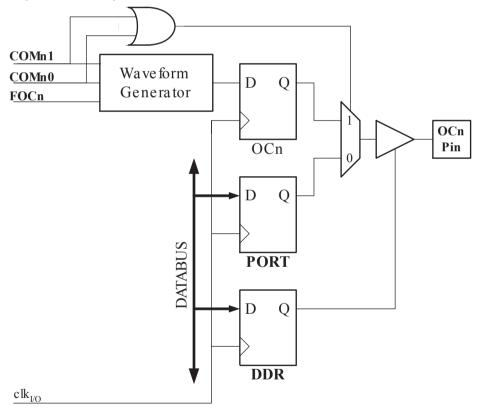
The general I/O port function is overridden by the Output Compare (OC2) from the waveform generator if either of the COM21:0 bits are set. However, the OC2 pin direction (input or output) is still controlled by the Data Direction Register (DDR) for the port pin. The Data Direction Register bit for the OC2 pin (DDR\_OC2) must be set as output before the OC2 value is visible on the pin. The port override function is independent of the Waveform Generation mode.
