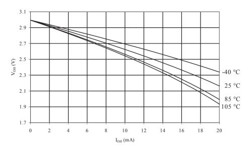
Figure 33-20 I/O Pin Output Voltage vs. Sink Current (V<sub>CC</sub> = 5V)
