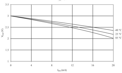
Figure 32-30 I/O Pin Output Voltage vs. Sink Current (V<sub>CC</sub> = 5.0V)
