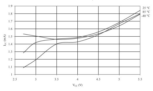
Figure 32-7 Active Supply Current vs. V<sub>CC</sub> (32kHz External Oscillator)
