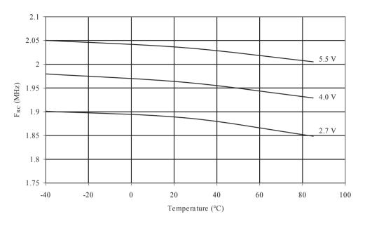
Figure 32-58 Calibrated 2MHz RC Oscillator Frequency vs.  $V_{CC}$
