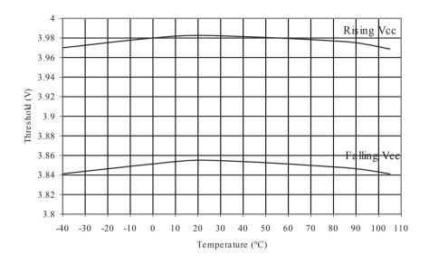
Figure 33-32 BOD Threshold vs. Temperature (V<sub>CC</sub> = 2.7V)
