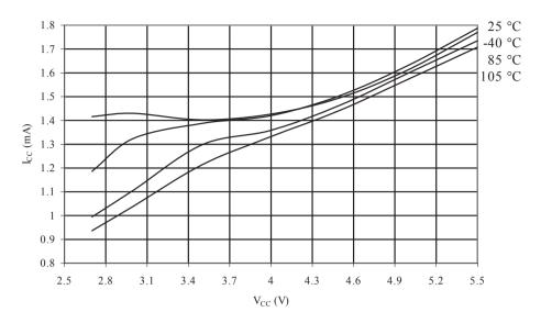
Figure 33-5 Active Supply Current vs. V<sub>CC</sub> (32 kHz External Oscillator)
