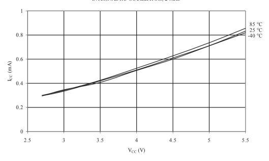
Figure 32-13 Idle Supply Current vs. V<sub>CC</sub> (Internal RC Oscillator, 1MHz)
