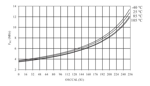
Figure 33-40 Calibrated 4MHz RC Oscillator vs. Temperature
