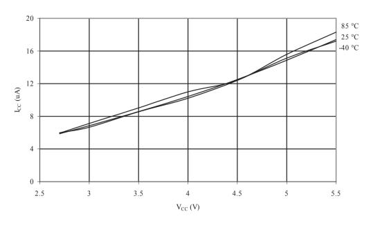
Figure 32-68 Analog Comparator Current vs. V<sub>CC</sub>
