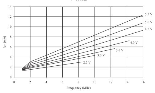
Figure 32-3 Active Supply Current vs. V<sub>CC</sub> (Internal RC Oscillator, 8MHz)
