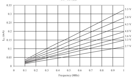
Figure 32-9 Idle Supply Current vs. Frequency (1 - 16MHz)
