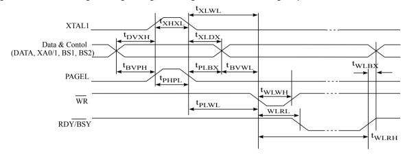
Figure 29-7 Parallel Programming Timing, Loading Sequence with Timing Requirements<sup>(1)</sup>
