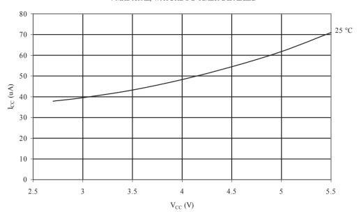
Figure 32-22 Standby Supply Current vs. V<sub>CC</sub> (6MHz Resonator, Watchdog Timer Disabled)
