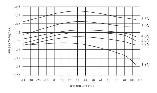
Figure 33-34 Bandgap Voltage vs. V<sub>CC</sub>
