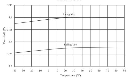
Figure 32-46 BOD Thresholds vs. Temperature (BOD Level is 2.7v)
