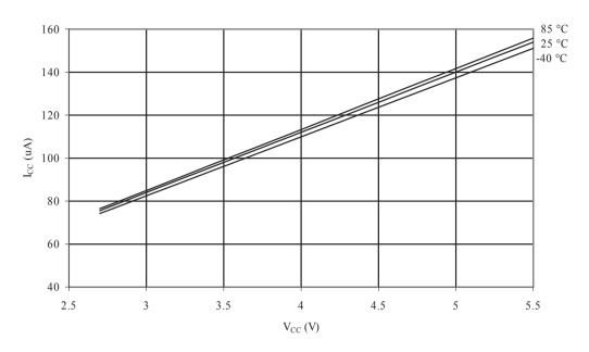
Figure 32-66 32kHz TOSC Current vs. V<sub>CC</sub> (Watchdog Timer Disabled)
