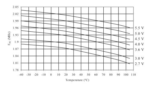
Figure 33-44 Calibrated 2MHz RC Oscillator vs. V<sub>CC</sub>
