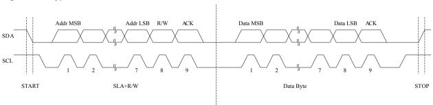
Figure 25-7 Typical Data Transmission
