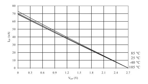
Figure 33-16 Reset Pull-up Resistor Current vs. Reset Pin Voltage (V<sub>CC</sub> = 5V)
