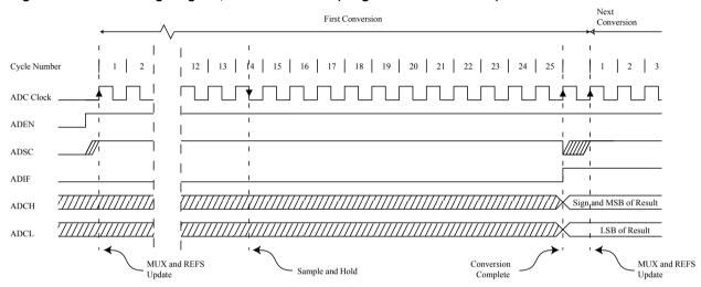
Figure 27-4 ADC Timing Diagram, Single Conversion
