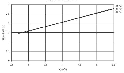
Figure 32-40 Reset Pin as I/O - Input Threshold Voltage vs. V<sub>CC</sub> (V<sub>IL</sub>, Reset Pin Read as "0")
