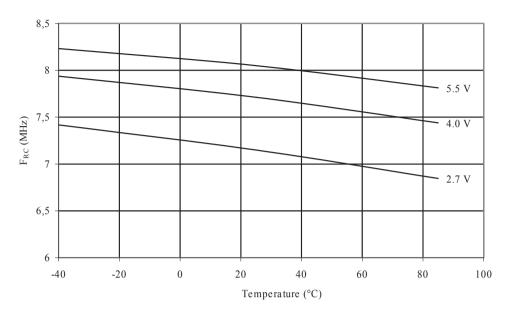
Figure 32-52 Calibrated 8MHz RC Oscillator Frequency vs.  $V_{CC}$
