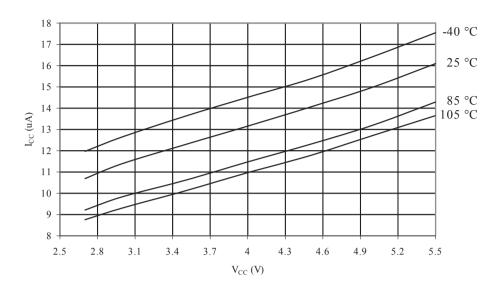
Figure 33-50 ADC Current vs. V<sub>CC</sub> (AREF = AV<sub>CC</sub>)
