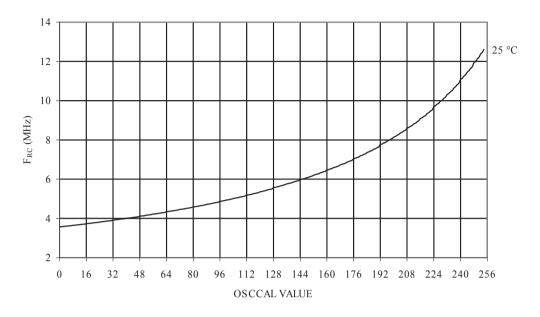
Figure 32-54 Calibrated 4MHz RC Oscillator Frequency vs. Temperature
