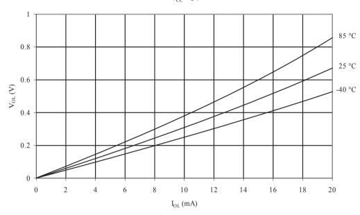
Figure 32-32 Reset Pin as I/O - Pin Source Current vs. Output Voltage (V<sub>CC</sub> = 5.0V)
