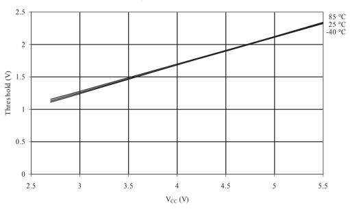
Figure 32-44 Reset Input Pin Hysteresis vs.  $V_{CC}$
