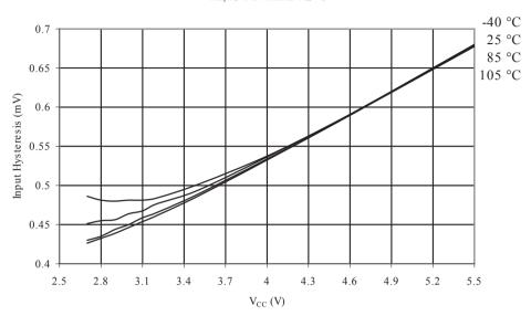
Figure 33-28 Reset Input Threshold vs. V<sub>CC</sub> (V<sub>IH</sub>, Reset Pin Read as '1')
