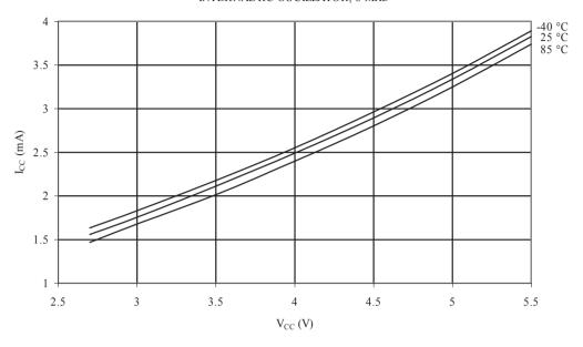
Figure 32-11 Idle Supply Current vs. V<sub>CC</sub> (Internal RC Oscillator, 4MHz)
