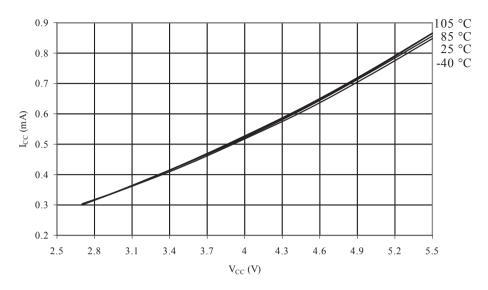
Figure 33-9 Idle Supply Current vs. V<sub>CC</sub> (Internal RC Oscillator, 1MHz)
