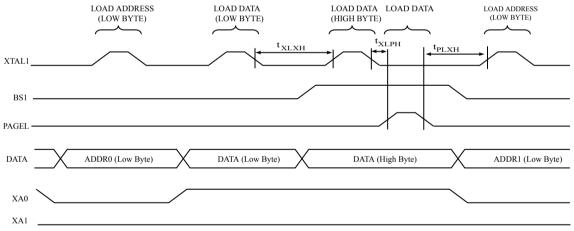
**Note:** 1. The timing requirements shown in the first figure in this section (i.e.,  $t_{DVXH}$ ,  $t_{XHXL}$ , and  $t_{XLDX}$ ) also apply to loading operation.
