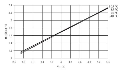
Figure 33-30 Reset Pin Input Hysteresis vs. V<sub>CC</sub>
