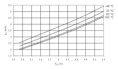
Figure 33-3 Active Supply Current vs. V<sub>CC</sub> (Internal RC Oscillator, 2 MHz)
