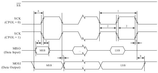
SPI interface timing requirements (Slave Mode)
