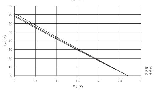
Figure 32-26 Reset Pull-up Resistor Current vs. Reset Pin Voltage (V<sub>CC</sub> = 5V)
