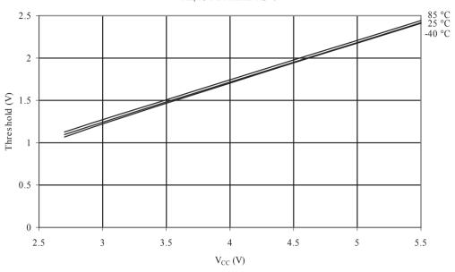
Figure 32-38 I/O Pin Input Hysteresis vs.  $V_{CC}$
