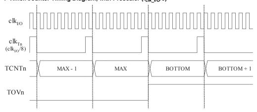
Figure 19-4 Timer/Counter Timing Diagram, with Prescaler (fclk I/O/8)
