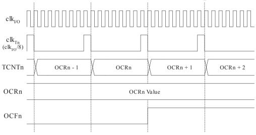
The figure below shows the setting of OCF2 and the clearing of TCNT2 in CTC mode.
