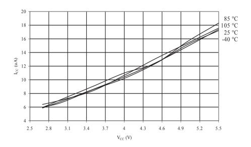
Figure 33-52 Analog Comparator Current vs. V<sub>CC</sub>
