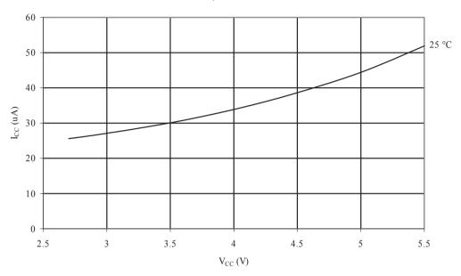
Figure 32-18 Standby Supply Current vs. V<sub>CC</sub> (1MHz Resonator, Watchdog Timer Disabled)
