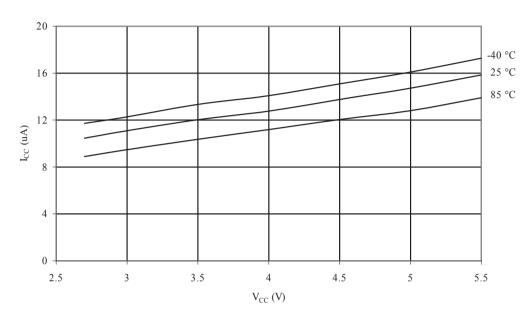
Figure 32-64 ADC Current vs.  $V_{CC}$  (AREF =  $AV_{CC}$ )
