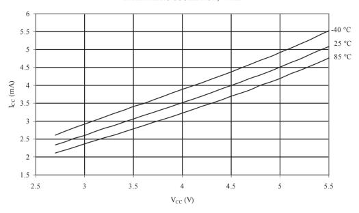
Figure 32-5 Active Supply Current vs. V<sub>CC</sub> (Internal RC Oscillator, 2MHz)
