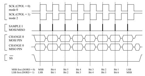
Figure 23-4 SPI Transfer Format with CPHA = 1
