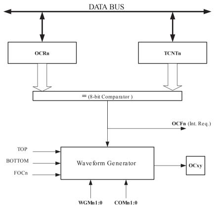
The OCR2 Register is double buffered when using any of the Pulse Width Modulation (PWM) modes. For the normal and Clear Timer on Compare (CTC) modes of operation, the double buffering is disabled. The double buffering synchronizes the update of the OCR2 Compare Register to either top or bottom of the counting sequence. The synchronization prevents the occurrence of odd-length, non-symmetrical PWM pulses, thereby making the output glitch-free.
