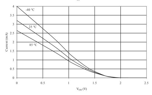
Figure 32-34 Reset Pin as I/O - Pin Sink Current vs. Output Voltage (V<sub>CC</sub> = 5.0V)
