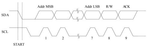
Figure 25-5 Address Packet Format
