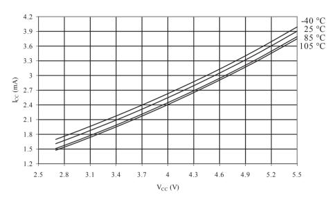
Figure 33-7 Idle Supply Current vs. V<sub>CC</sub> (Internal RC Oscillator, 4MHz)
