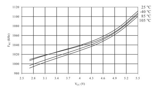
Figure 33-36 Watchdog Oscillator Frequency vs. Temperature
