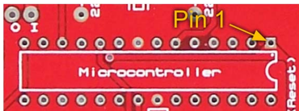
Figure 4. Microcontroller location on Board
