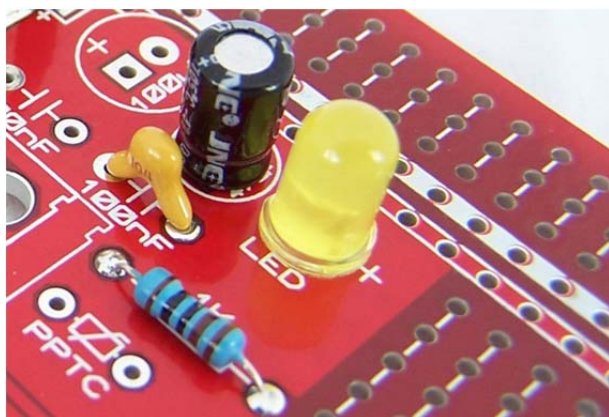
Figure 33. Vcc side capacitors
