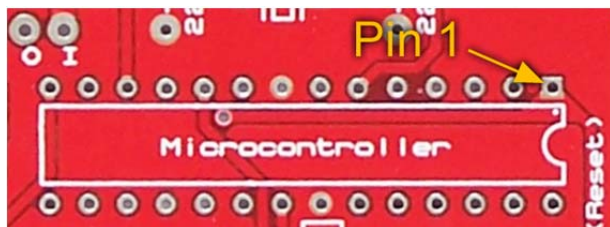
Figure 21. Microcontroller location on board
